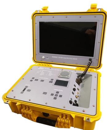
The HD-TVI video signal provides exceptional 1080p HD picture quality over cables in excess of 200 metres long. (Optionally, the camera can be supplied with an HD-AHD video output in place of HD-TVI)
