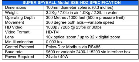
Spyballs are available in a number of configurations and with control options to suit a range of tasks from inspection to aquaculture - please visit our web site at www.submertec.co.uk to view these together with other Submertec products.
